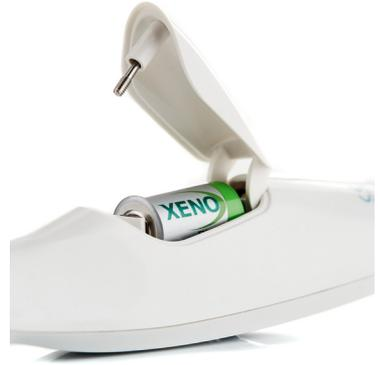
Figure 3.2 - Battery insertion
